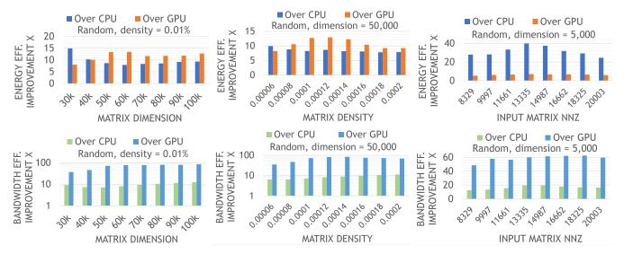
Fig. 12. Measured results over different matrices, showing energy and bandwidth efficiency of the proposed chip on uniform random matrices, normalized to a Core i7 CPU and V100 GPU running SpMM packages.
