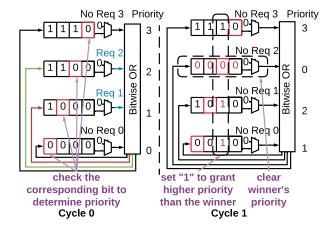
Fig. 7. LRG Scheme. The requesting nodes assert their priority bits and the winner is determined based on which requester receives a 0 in the corresponding response bit. The winner's priority bits are then cleared.
