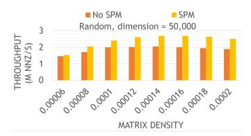
Fig. 11. Merge phase performance with and without scratchpad memory. Overall performance benefit of the scratchpad is 25.7%.
