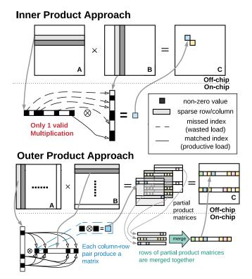
Fig. 1. High-level overview of SpMM using the inner-product and outer-product methods.
