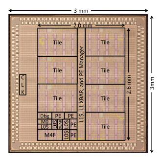
Fig. 9. Annotated 3.0-mm × 3.0-mm die photograph with GDS overlay. There are eight tiles per chip, each tile containing an ARM Cortex-M0, a Cortex-M4, and four PEs.
