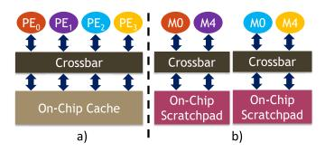
Fig. 3. High-level overview of the architectures suited for (a) multiply and (b) merge phases. Shared cache is suited for the predictable patterns in the multiply phase, whereas a private scratchpad is better for merge.
