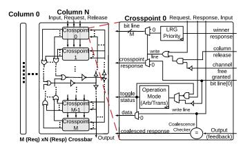
Fig. 6. OR trees of the SSN crossbar. Each crosspoint is one requester and the bitwise ORd results are sent back to each crosspoint.
