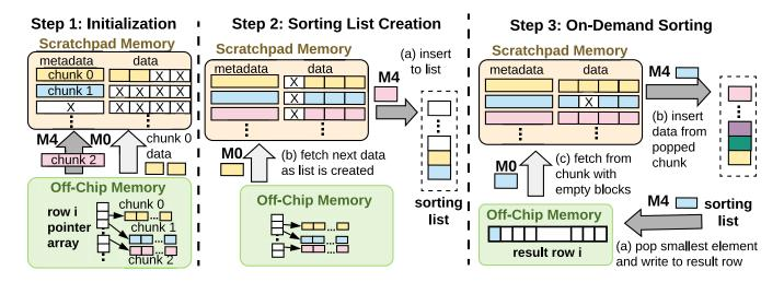
Fig. 4. Breakdown of the three steps of merge phase: initialization, sorting list construction, and on-demand sorting. M4 core performs the sorting operation on the data that have been loaded into the scratchpad by the M0 core.
