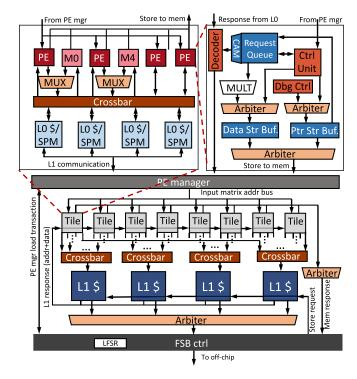
Fig. 5. Top-level diagram of the microarchitecture, a tile, and a PE. The chip contains a total of eight tiles, with each tile consisting of four PEs and a pair of M0 and M4 cores.
